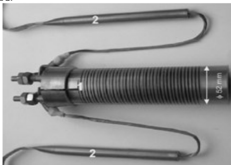
Figure 1: A sample made resistive fault current limiter
