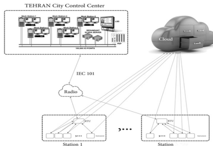
Fig. (5): The new model of cloud SCADA system
